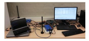
Figure 4: Setup of our interoperability test: the laptops on the left as well as the blue MK2 were used to transmit IEEE 802.11a/g/p frames, which have been received by the gray *Ettus USRP N210* in the middle.
