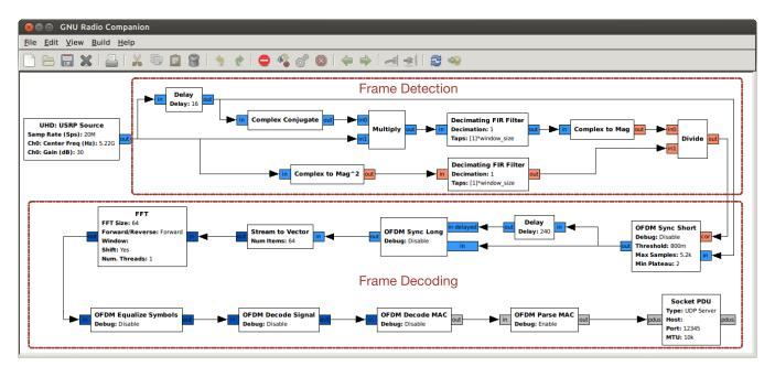
Figure 1: Overview of the blocks comprising the OFDM receiver in GNU Radio Companion.
