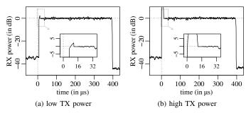
Figure 1. AGC delay when (a) increasing or (b) decreasing gain.
