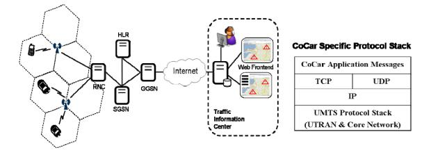
Fig. 4. CoCar specific Traffic Information Center and Protocol Stack
