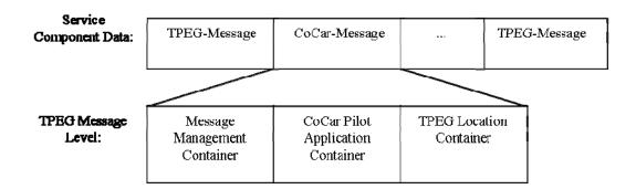
Fig. 2. Structure of a CoCar Message
