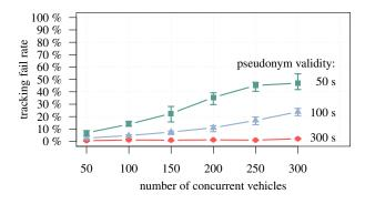
Figure 10: Chance of evading tracking in the blind-spot freeway scenario (beacon rate = 1Hz). Plotted are the averages over all simulation runs. Error bars extend from the 25% to the 75% quantiles.
