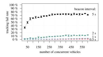
Figure 8: Chance of evading tracking in the synthetic grid scenario. Plotted are the averages over all simulation runs. Error bars extend from the 25% to the 75% quantiles.
