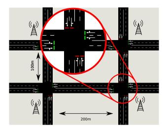
Figure 3: A grid scenario consisting of four intersections. Road segments leading to the intersections are 400 meters long. An adversary has placed 4 antennas and is able to fully monitor the scenario.
