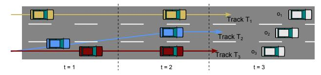
Figure 7: Tracking can be seen as the problem of assigning a new observation  $o_i$  to a track  $T_i$ .
