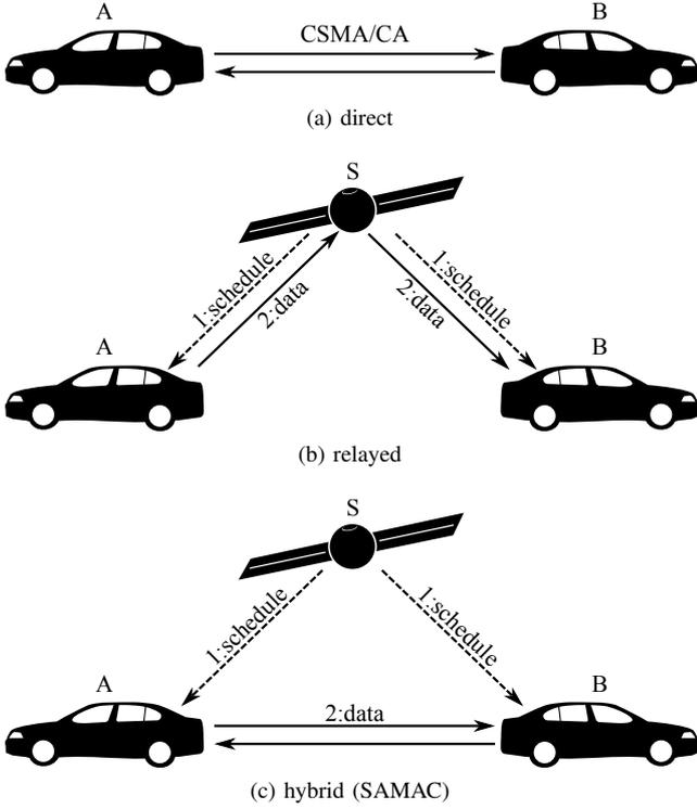
Figure 2. Different communication topologies considered in the evaluation.
