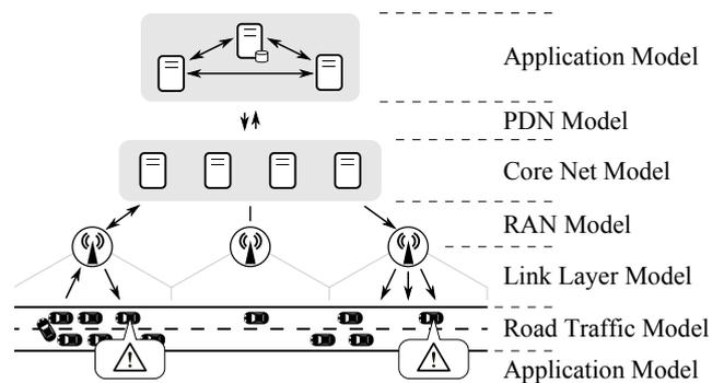
Fig. 1. Component model of the simulated UMTS-based Car-to-Infrastructure communication system
