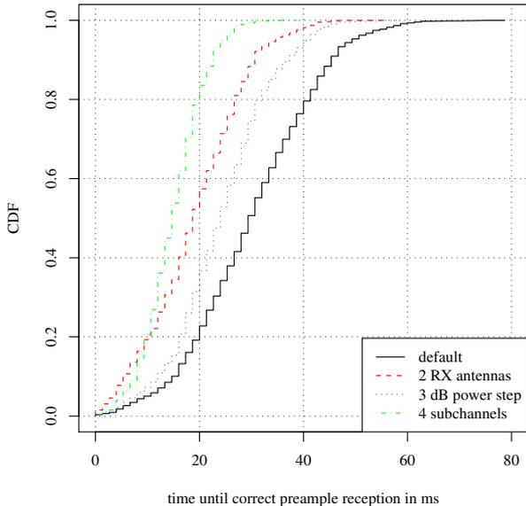
Fig. 4. CDF of the random access procedure duration for the default set of parameters ( $c_0 = -6$  dB, 2 dB power step, 1 RX antenna, 2 RACH subchannels), compared to alternative parametrizations
