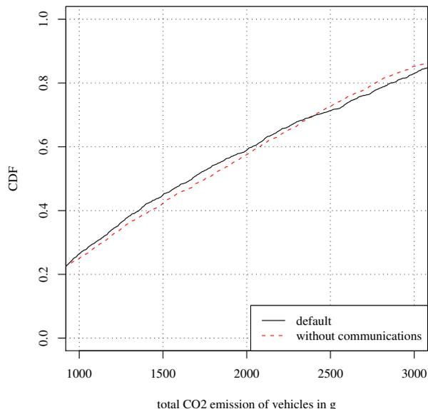
Fig. 7. Impact of the CoCar communication system on road traffic: Quantiles of vehicles' CO<sub>2</sub> emissions.
