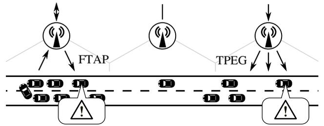
Fig. 2. Protocols used in the CoCar communication system
