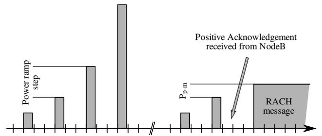
Fig. 3. Access procedure on RACH: One failed, one successful attempt
