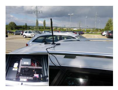
**Figure 3.12** – Position of the shark fin antenna assembly, omnidirectional antenna, and GPS receiver used for signal attenuation measurements; inset: installation of the DENSO WSU 802.11p radio in the trunk.
