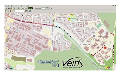
**Figure 3.5** – Screenshot of the running simulative prototype. A contiguous stream of vehicles, leaving the campus and heading to a business park, is interrupted by a traffic obstruction at point ①. Dynamic re-routing has started.
