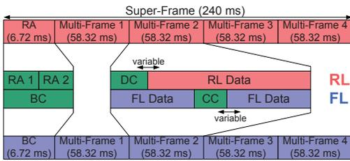
Fig. 1. L-DACS 1 frame structure
