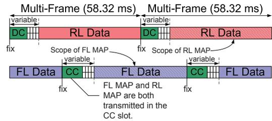
Fig. 2. L-DACS 1 resource allocation structure
