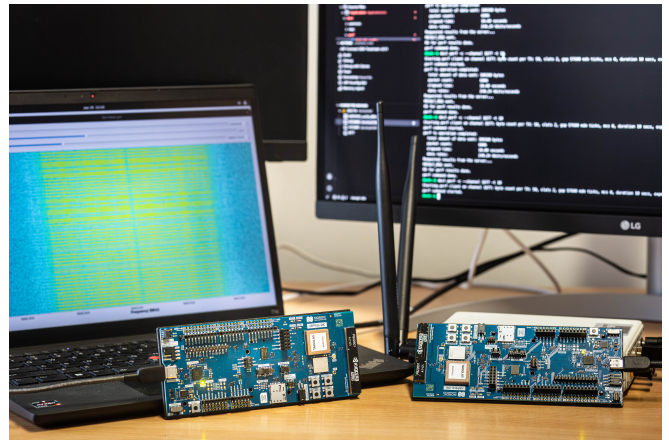
Figure 8. Experimental setup of two nRF9151 DK and an Ettus USRP B210 Software Defined Radio (SDR) doing a throughput test. The SDR is capturing the signal and plotting a spectogram with GNU Radio.
