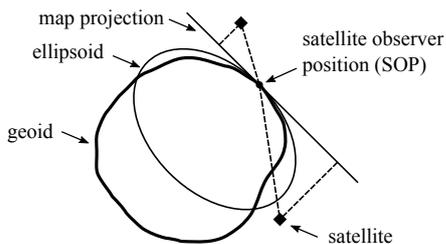
Figure 1. Satellite Observer Position (SOP) centric approach.
