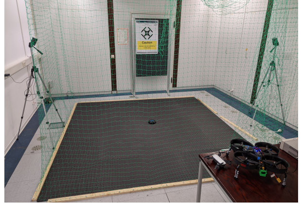
Figure 1. Measurement setup using HTC Vive base stations. The base stations are mounted on tripods and at a height of 1.6 m. The total flight space has a size of 3 m x 3 m.
