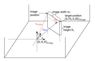
Figure 3: Illustration on how 3D coordinates can be extracted from 2D image coordinates in Unity
