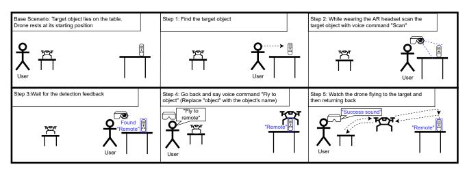
Figure 1: Example use case scenario for an intelligent aerial assistant. The manual scanning step may be removed in the future for even more automation.
