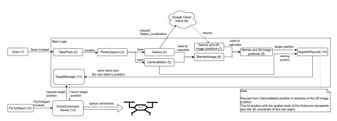
Figure 2: Workflow from giving speech inputs to the UAV approaching the chosen destination.
