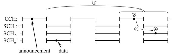
Figure 2: MCB operation in four steps: (1) coarse-grained interval selection, (2) selecting a time for the announcement, (3) selecting a channel and time for the data and sending an announcement, and (4) sending the data.
