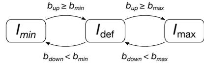
Figure 4: State diagram of a transmit rate control algorithm. The beacon interval (defined in the three states) changes according to the channel busy ratio. The transition is performed if the busy ratio is over or under a threshold for a given time interval.
