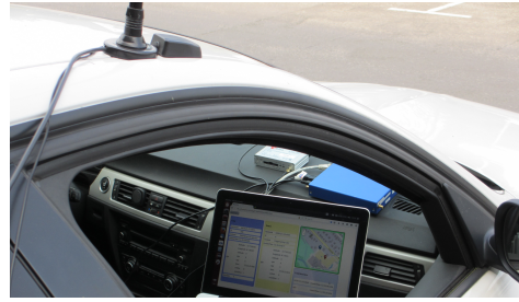
Figure 2. Hardware setup for the field test: OpenC2X is running on a small Linux PC in the car; for the GPS receiver and the WLAN card one antenna each is mounted on the roof.
