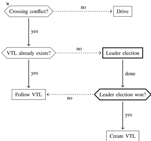
Figure 1. The basic Virtual Traffic Light (VTL) flow. It depicts what steps a single car has to perform when participating in the algorithm.
