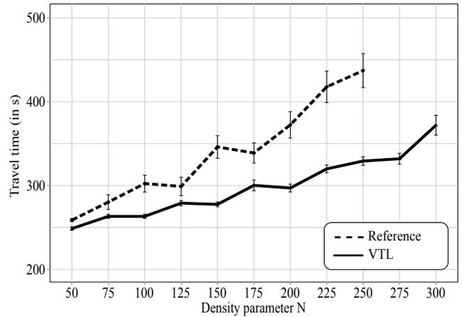
Figure 4. Travel time of cars for various traffic densities, drawn for Virtual Traffic Lights (VTL) and for physical traffic lights (reference). Also shown is the 95% confidence interval. There are no data points for  $N = 275$  and  $N = 300$  in case of the reference traffic lights because for these density we experienced vehicles waiting for longer than 1000 s. Such a long inactive time does not make sense for a realistic simulation and shows that VTL is able to handle a higher density.
