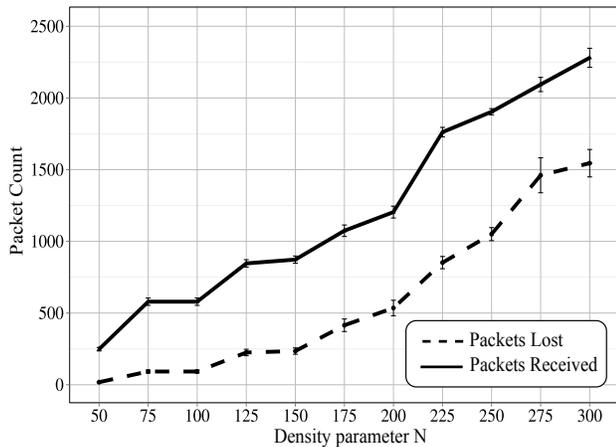
Figure 6. Received broadcasts and lost packets during the simulation, plotted for different density parameters  $N$ .
