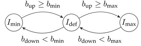
Fig. 3. State machine of the TRC algorithm.
