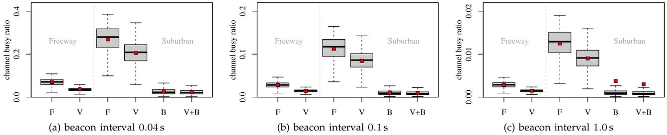
Fig. 6. Beacon performance (channel busy ratio) of static beaconing for the different radio shadowing scenarios.
