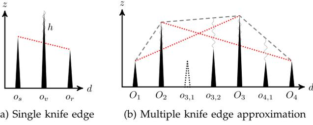
Fig. 2. Approximation of signal power loss by moving vehicles.
