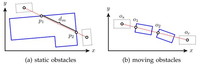
Fig. 1. Calculation of line of sight intersection points with buildings and vehicles, cast as a *red and blue line segments* intersection problem.
