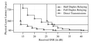
Figure 3. Computed Physical Layer Latency (PLL) in the considered scenarios of Half Duplex Relaying (HDR), Full Duplex Relaying (FDR), and Direct Transmission (DT).
