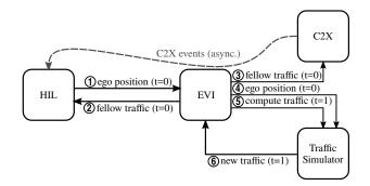
Figure 2. Flow and order of exchanged messages among simulator components. Synchronous message cycles (1 to 6) repeat every 100 ms. C2X event messages relevant for the ego vehicle are sent asynchronously in the moment they occur.
