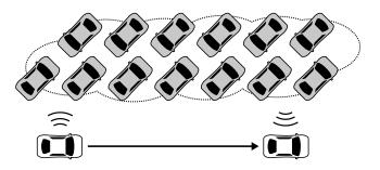
Figure 1: A schematic overview of our approach where a driving car passes a cluster of parked cars forming virtual network infrastructure. The physical connection is automatically handed over among cars in the cluster as the driving car passes by.
