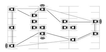
Figure 2: Outline of the proposed algorithm for gateway selection. First, the convex hull is computed (dashed line). Second, additional nodes are added based on the concave hull (solid line). Third, based on Algorithm 1, the gateway selection is performed.
