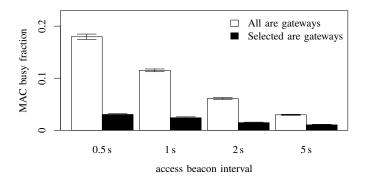
Figure 6: Fraction of time the MAC is observed busy in the artificial scenario. Shown are different access beacon intervals for s active gateway selection as well as for the baseline option where all parked cars act as gateways.
