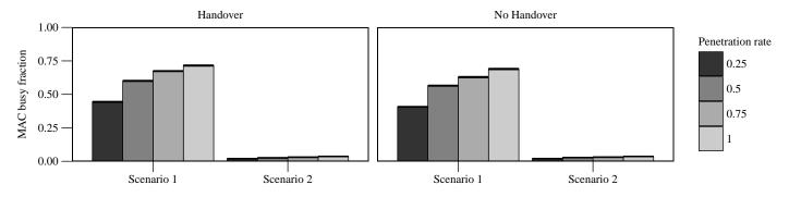
Figure 13: MAC busy fraction when streaming 1 kByte every 0.05 s in both scenarios for various penetration rates including 95% confidence intervals.
