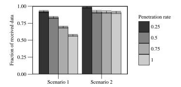
Figure 10: Fraction of successfully transmitted data (512 kByte) in both scenarios and different penetration rates including 0.95% confidence intervals.
