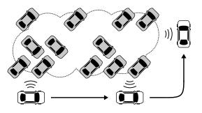
Figure 1: Schematic overview of our concept, where a driving car passes a cluster of parked cars forming virtual network infrastructure. The physical connection is handed over among gateways in the cluster as the driving car passes by.
