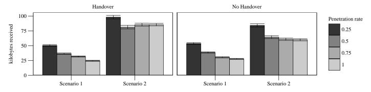
Figure 12: Amount of received streaming data (0.25 kByte every 0.2 s) in both scenarios and different penetration rates including 0.95 % confidence intervals.
