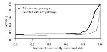
Figure 9: Fraction of data successfully transferred data between the sender (parked car) and the receiver (moving car requesting the data). We also distinguish between all cars act as gateways and the gateway selection algorithm.
