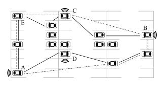
Figure 3: Outline of the proposed algorithm for gateway selection. First, the convex hull is computed (dashed line). Second, additional nodes are added based on the concave hull (solid line). Third, based on Algorithm 1, the gateway selection is performed.
