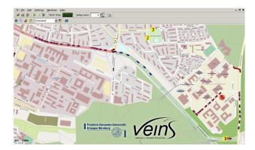
Fig. 2. Screenshot of the running simulative prototype. A contiguous stream of vehicles, leaving the university campus and heading to a business park, was interrupted by a traffic obstruction at point <sup>①</sup>. Dynamic re-routing has started.
