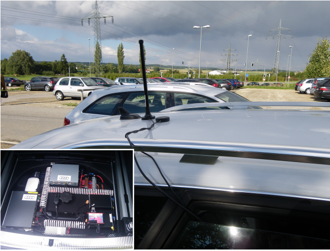
Figure 2. Position of the shark fin antenna assembly, omnidirectional antenna, and GPS receiver on the roof; installation of the DENSO WSU 802.11p radio in the trunk (inset).
