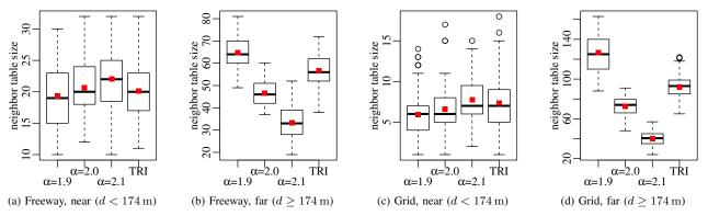
Figure 6. Distribution of nodes' neighbor table sizes (considering either only near or far neighbors). Results from the 1D Freeway and 2D Grid scenarios (1 Hz beacon interval), plotted for three empirical adaptations of the Free-space path loss model, as well as for the Two-Ray Interference model.
