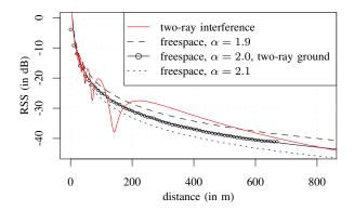
Figure 5. Model comparison for the Free-space model using different  $\alpha$  values and the Two-Ray Interference model. For  $d_c < 866.6$  m, results for  $\alpha = 2.0$  and for the simplified Two-Ray Ground model are identical.
