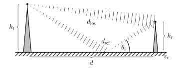
Figure 1. Conceptual model of ground reflection causing distance-dependent constructive and destructive signal interference effects at the receiver.
