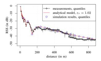
Figure 4. Measurement results of received signal strength vs. distance between sender and receiver (median, 1%, and 99% quantiles), overlaid with the calibrated Two-Ray Interference model and simulation results.
