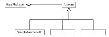
Fig. 6 Overview of the newly added antenna classes.
