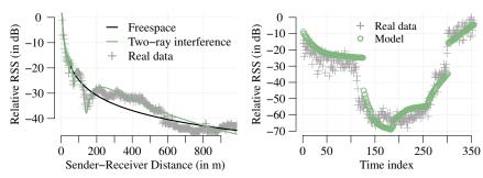
(a) Real-world measurements compared to the (b) Real-world measurements compared to the free-space model and the two-ray interference obstacle model in 2 based on [55] model based on [52]
