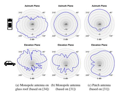
**Fig. 5** Azimuth and elevation planes of exemplary vehicular antenna patterns. The gain is given in dBi.
