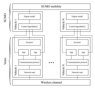
Fig. 11 High-level architecture of PLEXE components.
